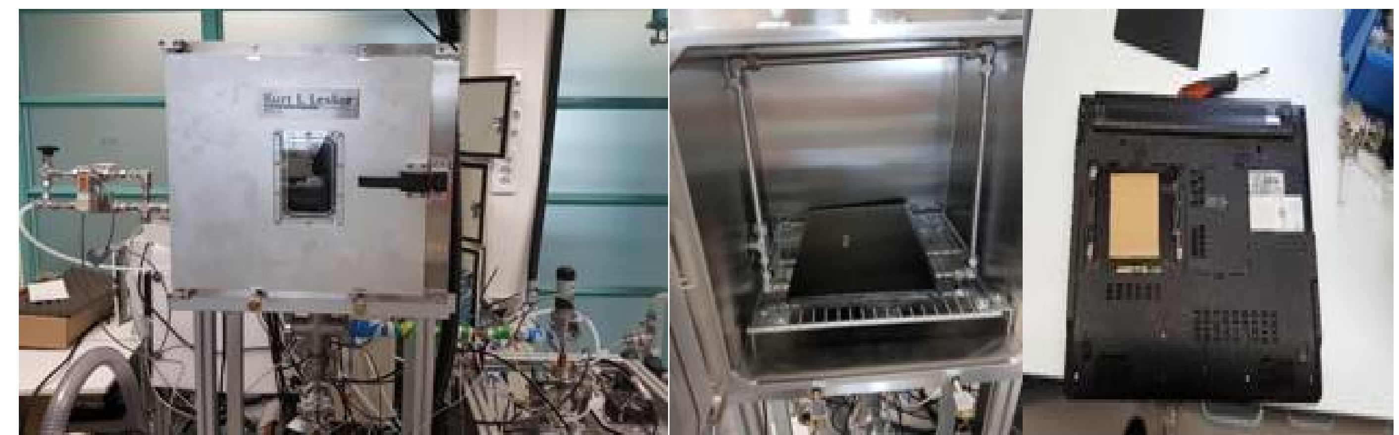
Figure 2: (left) Proof of concept system consisting of a vacuum chamber, pressurization system and CI inlet to Tarkka TOF. (middle) Laptop in the sample chamber. (right) simulated explosives threat (Explosives deposited on cardboard or aluminum foil) placed inside laptop for detection
