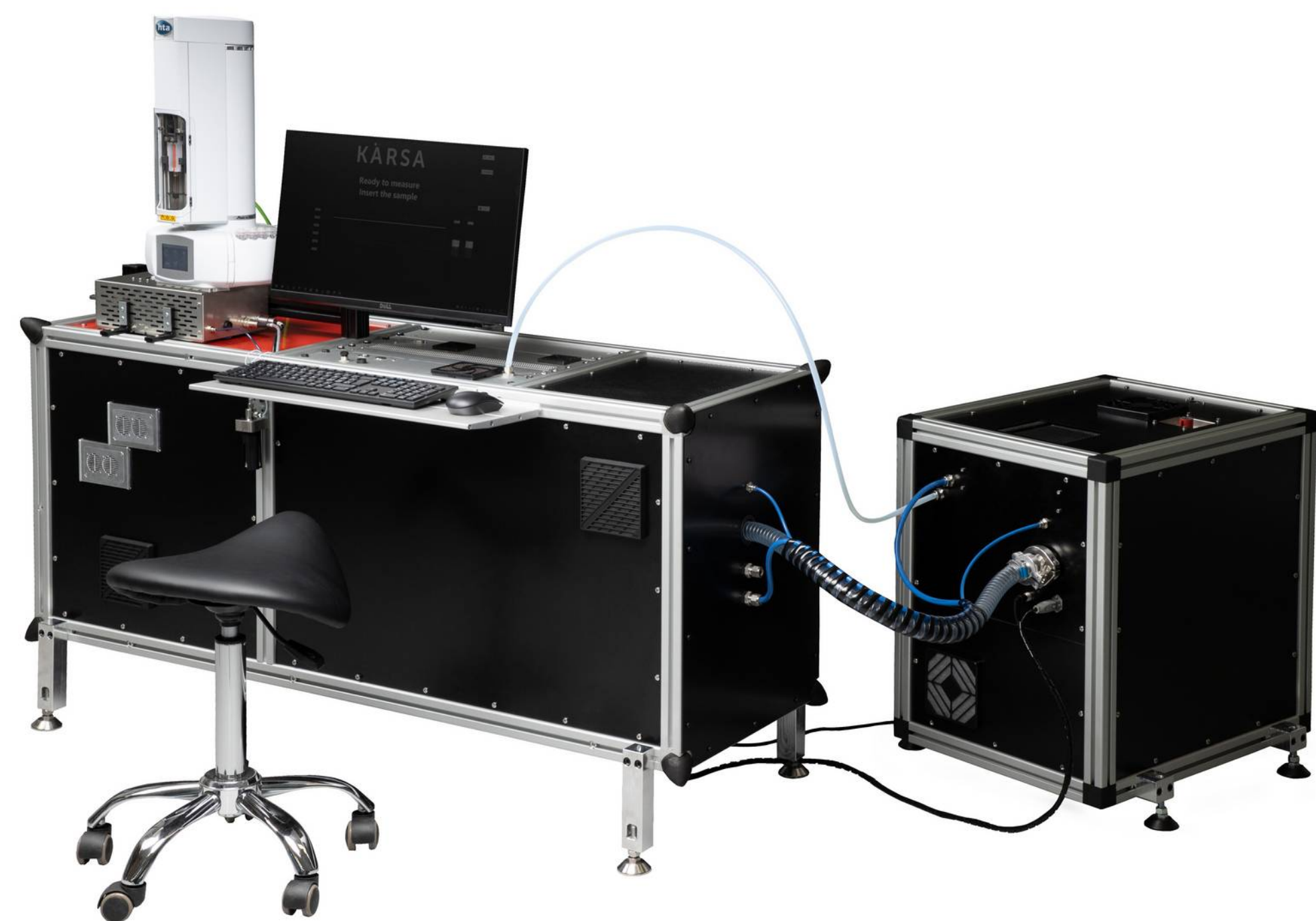
Figure 1: Tarkka TOF consists of the high resolution (resolving power~10000) time of flight mass spectrometer (TOF-MS), the atmospheric pressure interface (API) and the Chemical Ionization inlet. The dimensions are 148cm x 62cm x 48cm and weight is 110kg, and a separate pump rack.
