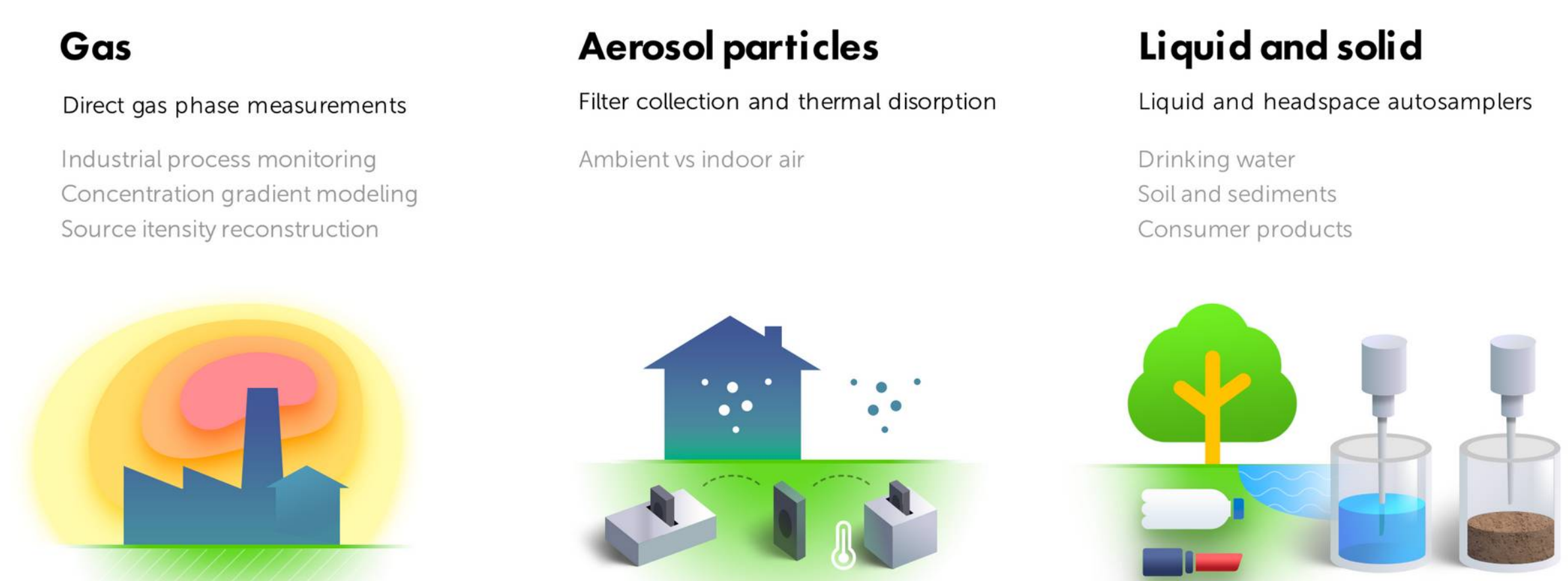
Figure 4: The Tarkka TOF allows the direct, online analysis of threat molecules, collection of vapours and particles on filters and subsequent desorption, and analysis of liquid samples.
